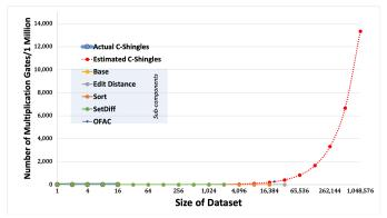
Fig. 6: Number of multiplication gates in the circuit for searching for a particular string of length 30 in a dataset. The x-axis is the number of points in the dataset and the y-axis is the number of multiplication gates in the compiled circuit.
