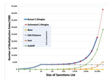
Fig. 5: Circuit size for proving that a 30-character string is not in a sanctions list using jsnark. The x-axis is the number of points in the list and the y-axis is the number of gates in the circuit. Edit distance is calculated on the first 15 words that constituted c-shingle matches.
